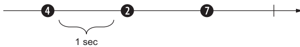
Figure 9.4 The unidirectional flow of an observable is depicted as an arrow. You can think of the producer and subscribers (not shown but implied) as being on the left and right sides, respectively. Events (marbles) move across the observable.
