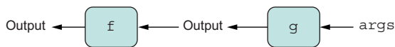
Figure 4.3 High-level diagram of composition. The directions of the arrows are important. Composition works right to left. So in f composed with g , g receives the initial input arguments. Then g 's output is input to f . Finally, f 's result becomes the output of the entire operation.
