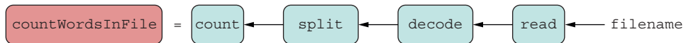
Figure 4.5 The logic of countWordsInFile derives from the logic of composing other single-responsibility functions such as read , decode , split , and count .
