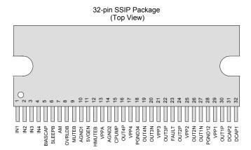
Note: The heat slug of the TA2041 is connected to PGND.
