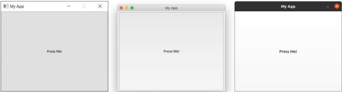
Figure 6. Our fixed-size window, notice that the maximize control is disabled on Windows & Linux. On macOS you can maximize the app to fill the screen, but the central widget will not resize.
