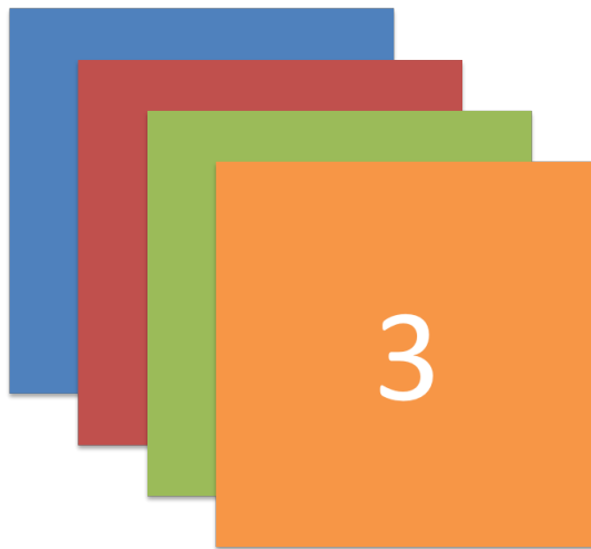
Figure 29. QStackedLayout — in use only the uppermost widget is visible, which is by default the first widget added to the layout.
