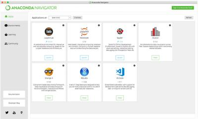
Figure A.8 Anaconda Navigator home screen Click the Environments tab on the left menu to display a list of all environments. Select a conda environment to see its installed packages, including their descriptions and version numbers.
