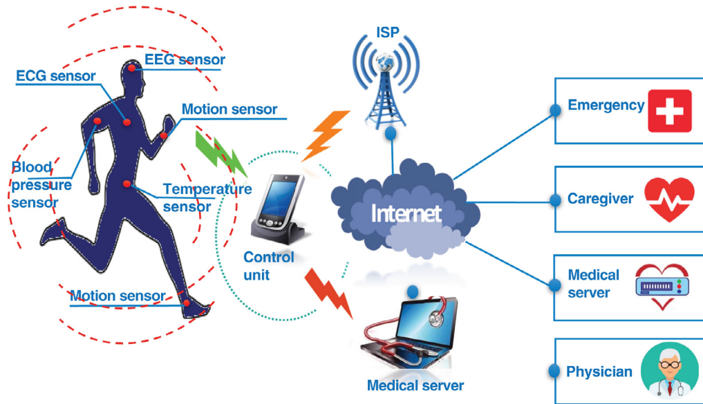
FIGURE 4.9 The general experimental setup for smart healthcare monitoring systems (SHMS). Source: Adapted from Subasi et al. (2020b).
