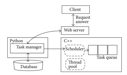
Figure 3: Active object implementation delivered by the framework. The client requests are transformed into commands automatically, which are executed by separate threads.
