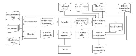
Figure 1: Platform architecture, receiving high-level code.
