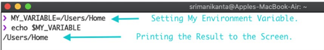
Figure 5-6. Creating environment variable using CLI
