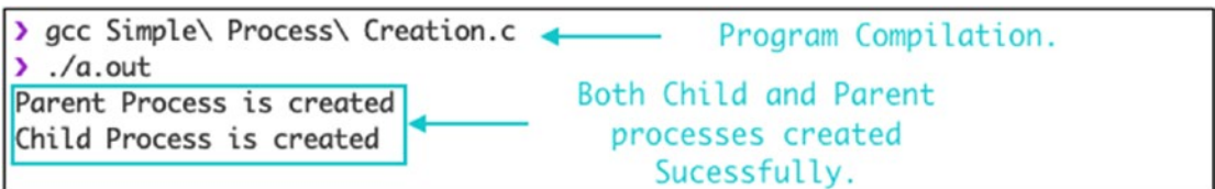
Figure 5-14. Output of the program on process creation using C
