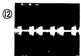
⑫ IC303 Pin 15 PB MODE 629KHz COLOR INPUT SIGNAL
