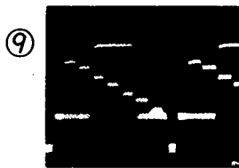
⑨ IC303 Pin 3 PB MODE 3M LPF OUTPUT SIGNAL
