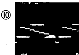
⑩ IC303 Pin 10 PB MODE 1H DELAY OUTPUT SIGNAL
