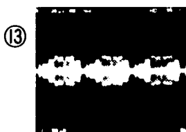
⑬ IC303 Pin 25 PB MODE 3.5MHz MAIN CONVERTER OUTPUT SIGNAL
