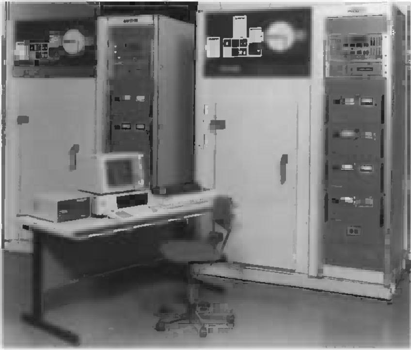
**Figure 7.** Air ambient burn-in system. (Courtesy Aehr.)
