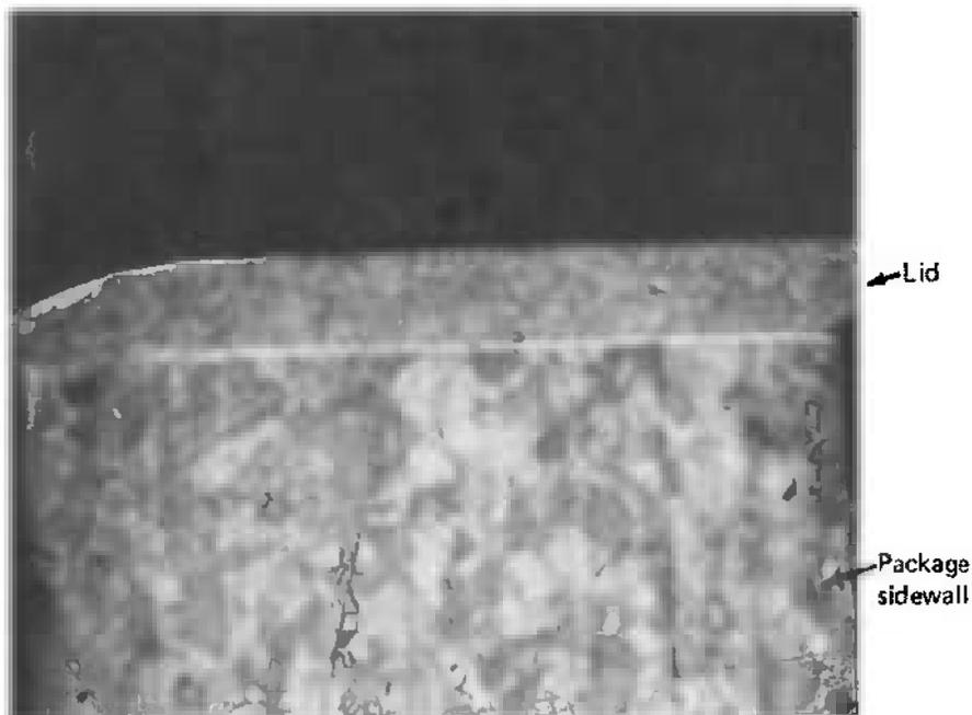
**Figure 49.** Cross-section of lid-package seam weld joint (100x). (Courtesy of Rockwell International.)
