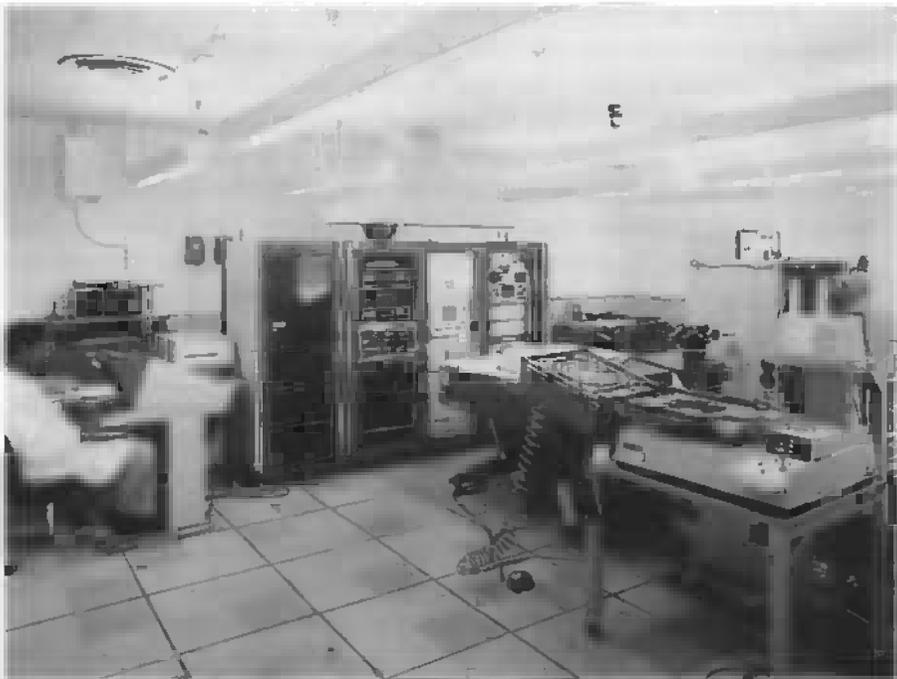
**Figure 2.** Automated electrical test equipment—Tektronix 3260. (Courtesy of Rockwell International.)
