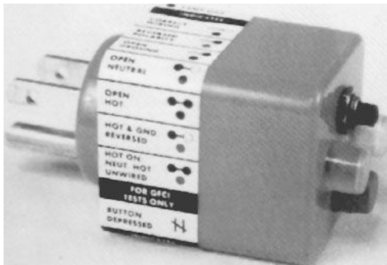
FIGURE 5.14 A typical receptacle tester. (Courtesy ETCO Corp.)
