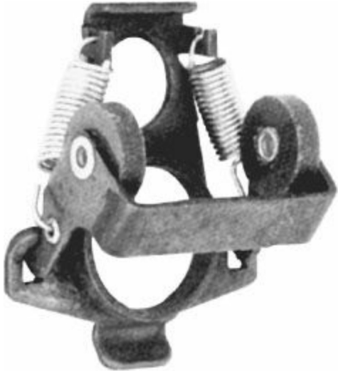
FIGURE 3.6 Typical centrifugal mechanism assembly of a centrifugal switch. (Courtesy Franklin Electric Co.)
