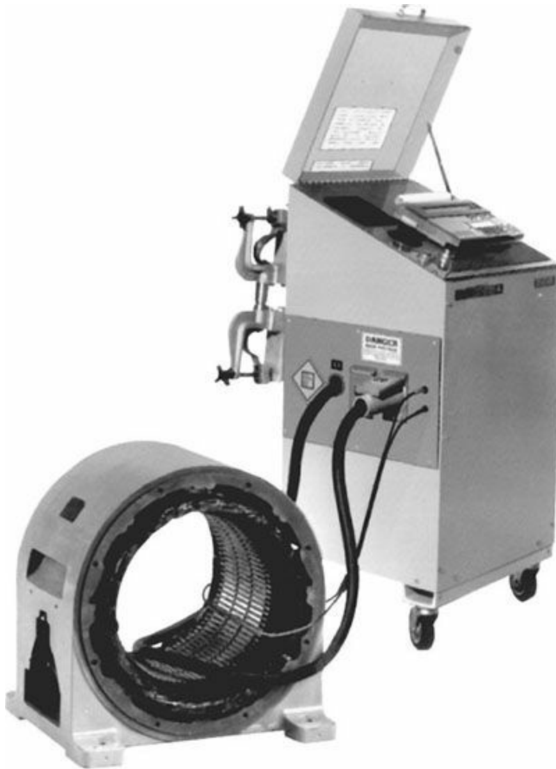
FIGURE 3.40 A setup procedure for measuring core losses using a core loss tester. (Courtesy Lexseco, Inc.)
