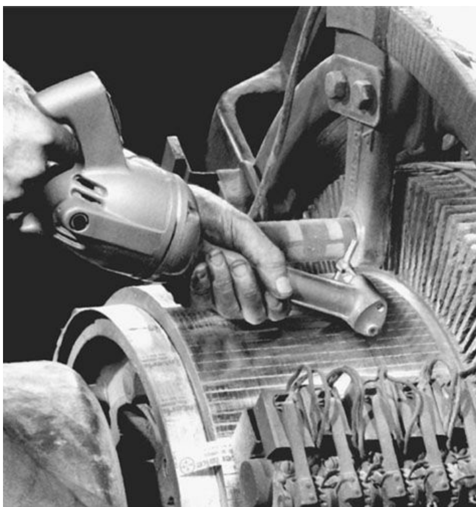
FIGURE 3.36 Removing mica from the commutator slots with a direct-drive mica undercutter. (Courtesy Ideal Industries, Inc.)
