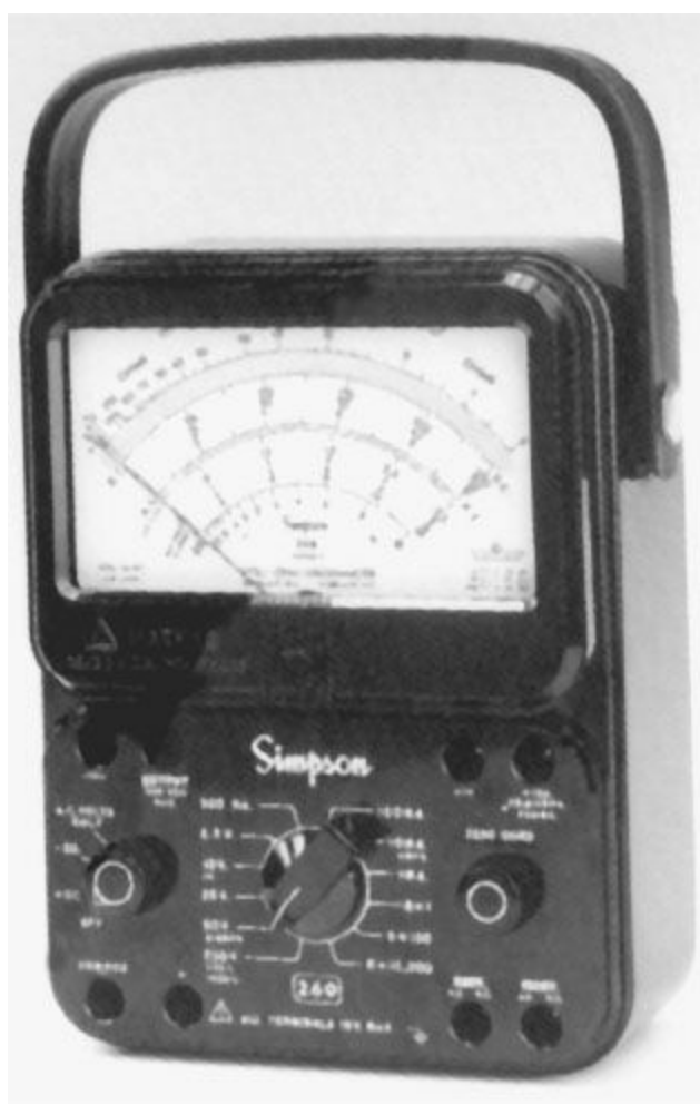
FIGURE 2.1 A typical VOM. (Courtesy Simpson Electric Co.)
