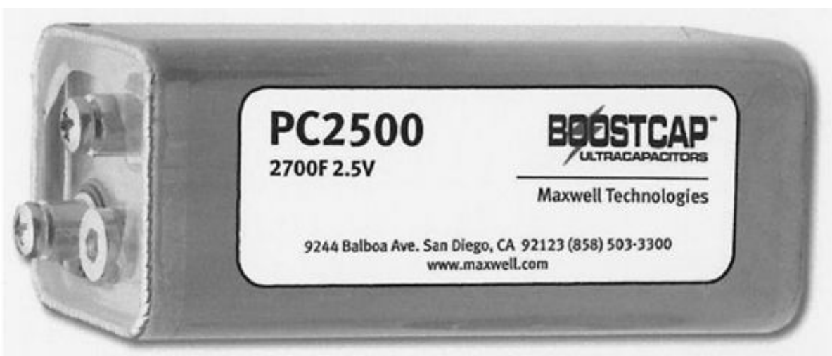
FIGURE 1.37 A 2700-F ultracapacitor. (Maxwell Technologies.)
