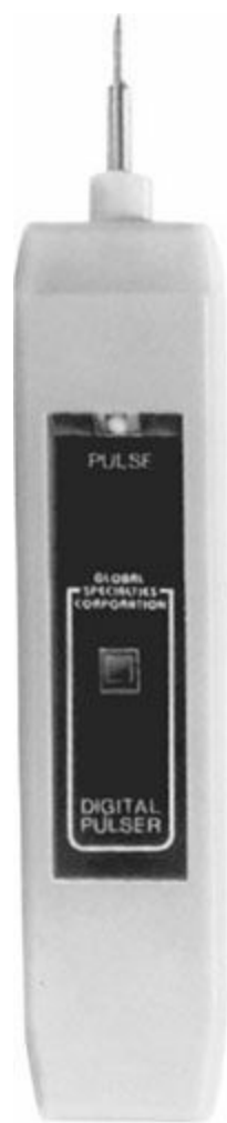
FIGURE 2.13 A handheld digital logic pulser. (Courtesy Global Specialties Corp.)
