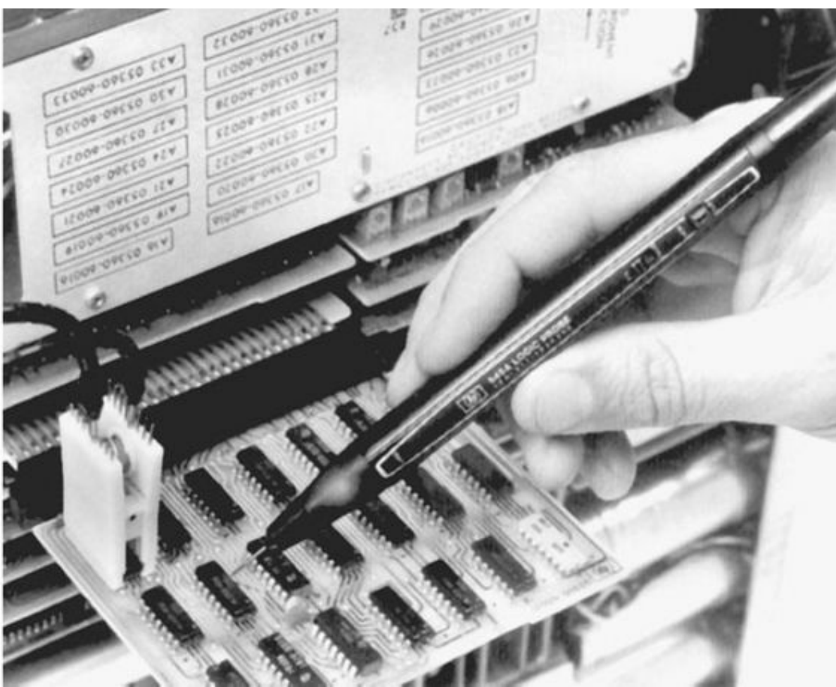
FIGURE 1.35 Using a logic digital IC probe to test an IC. (Courtesy Hewlett-Packard.)
