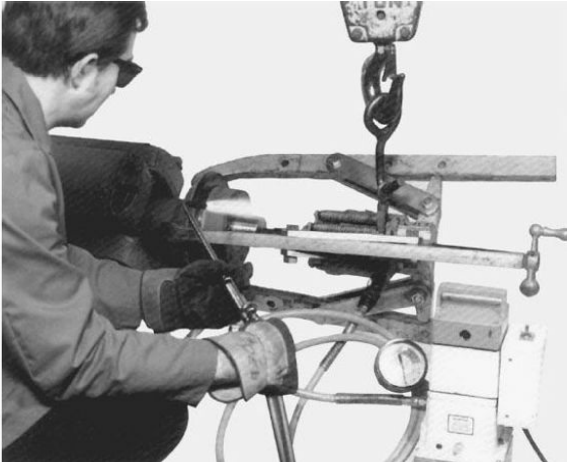
FIGURE 3.44 Removing a bearing with a bearing puller and heat. (Courtesy Marathon Electric.)
