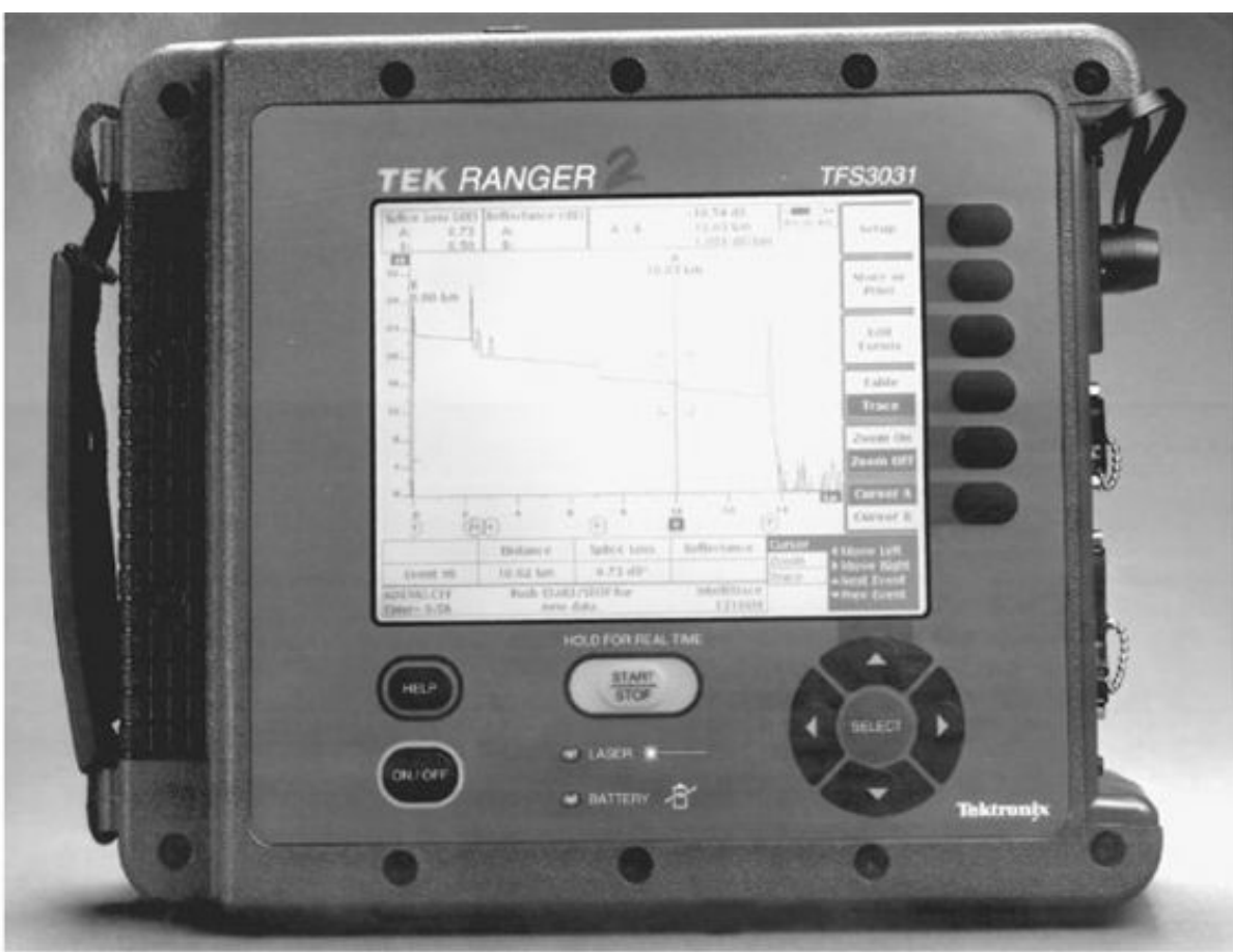
FIGURE 2.16 An optical time-domain reflectometer (OTDR). (Courtesy Tektronix, Inc.)
