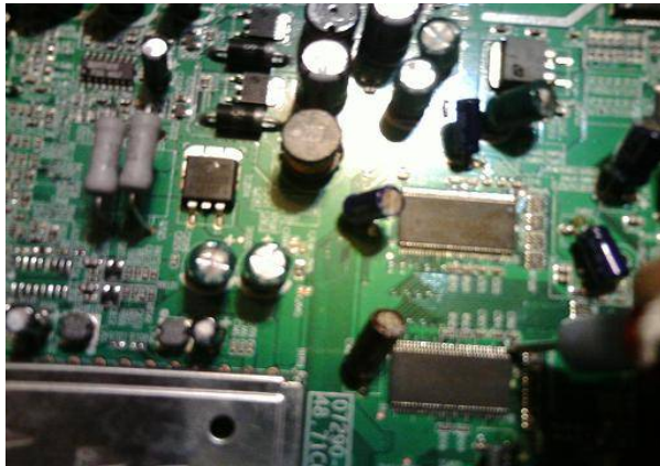
Checking Positive Supply Voltage Pin Of A NAND Memory IC
