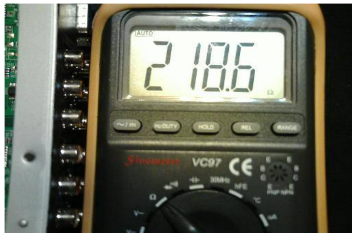
Meter Reading 218.6 ohms the resistor stated 220 ohms on the side and at 5% tolerance so this as a good resistor
