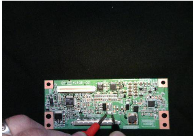
Checking controller board pico fuse
