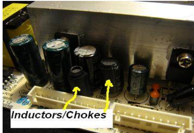
Inductors In Secondary Side Of PSU
