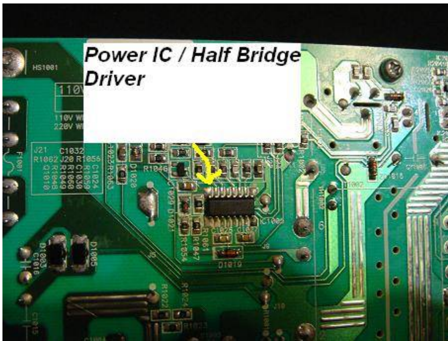
Bottom of PSU showing SMD power IC/half bridge driver
