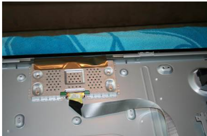
Cable from main board to controller board
