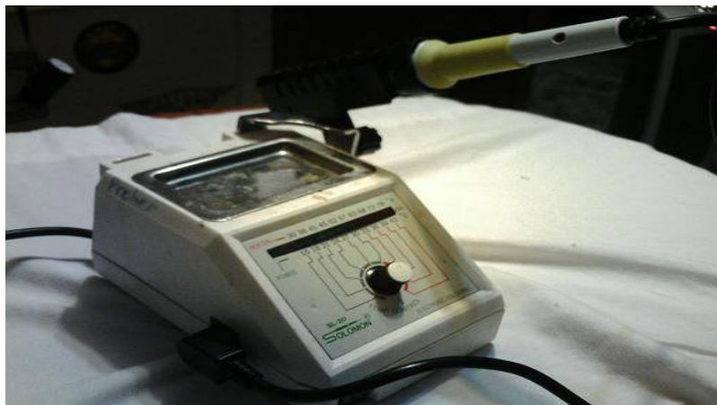
Variable temperature soldering station with LED display
