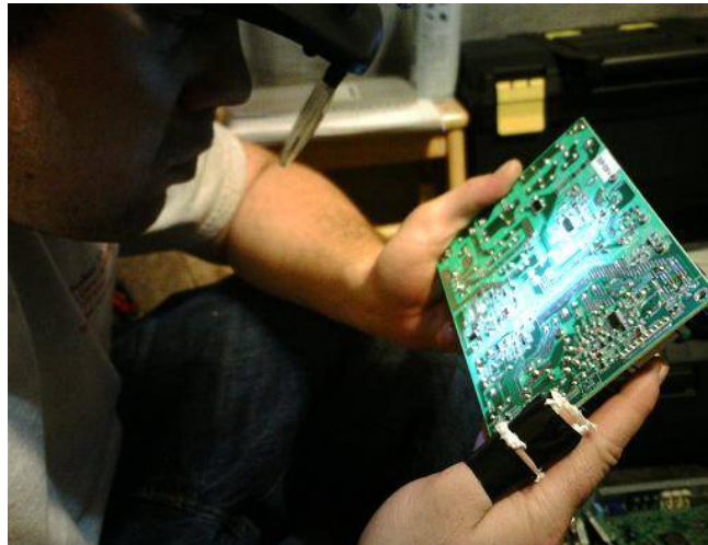
Inspecting PCB For Bad Solder Connections
