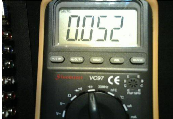
Meter Reading in nF(nanofarads) 0.052 nanofarads or 52 picofarads
