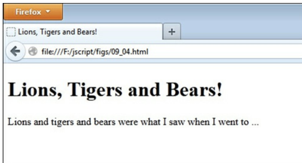
Figure 9-4 The title of the document is shown as a heading on the page.
