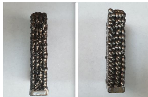
Figure 3. The model of the "real" situation of layer deposition obtained through GMAW standard(left) and GMAW CMT(right) techniques.
